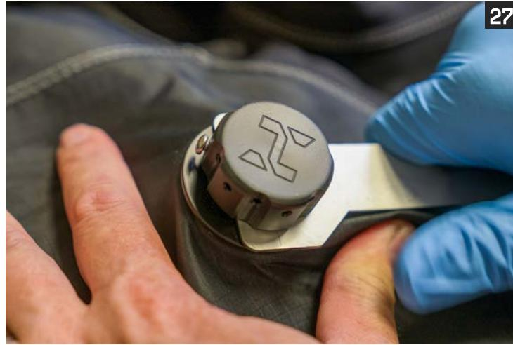
27. This same pressure can be applied from the top of the suit as long as you trap the hose into place to keep the bottom assembly from rotating.
