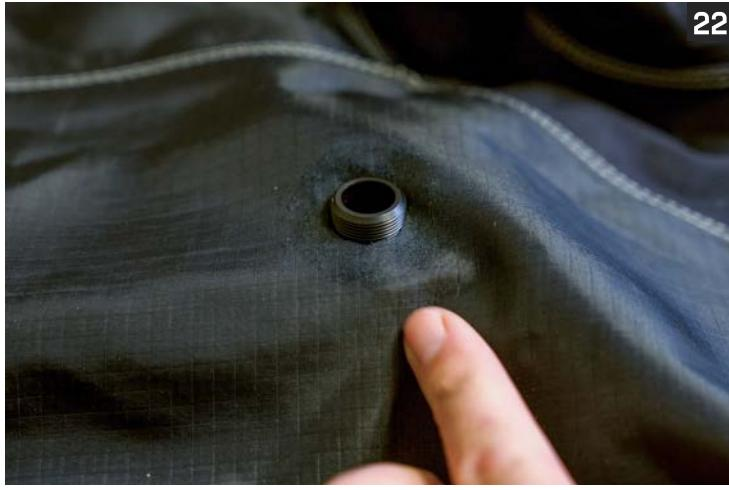
22. Rotate the base of the P-Valve slightly to get the desired angle. Angle of the hose should travel towards the top edge of the drysuit pocket.
