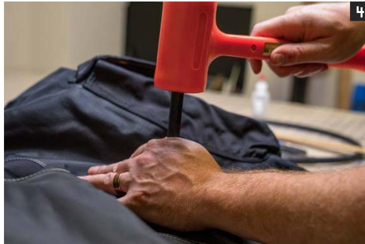
4. Using a Rubber mallet, strike the punch the desired times to get through the fabric.
