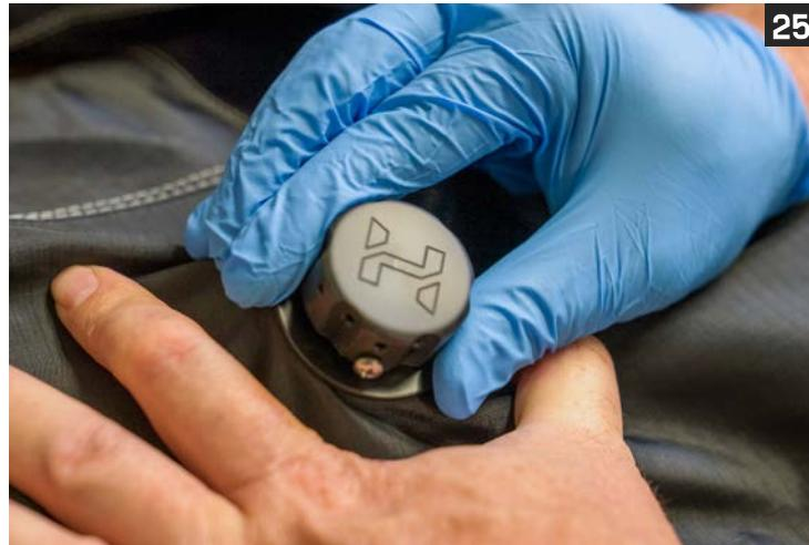
25. Using finger tight assembly, make sure the base of the valve is tightened and secured. Do not just screw down the cap portion of the assembly.
