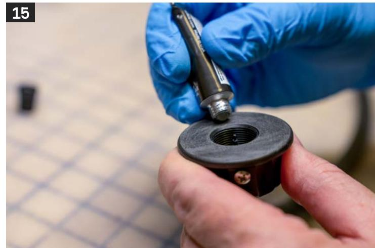
17. Apply same bead and strategy to the opposing end of the P-Valve. These will allow bonding to the suit and prevent leaks.
